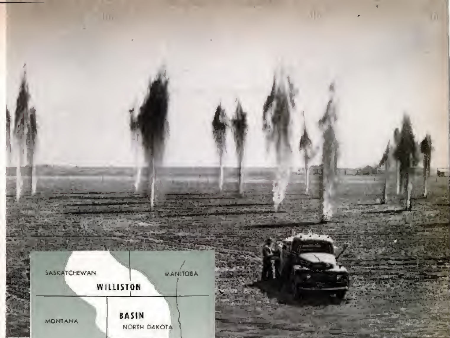
Thunder in the "back forty"—as survey crew explodes dynamite charges and measures the ground echoes with instruments to learn the nature of underlying rock
